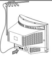
Connect aerial to aerial jack. It is usually connected by means of a 75 ohm cable.
